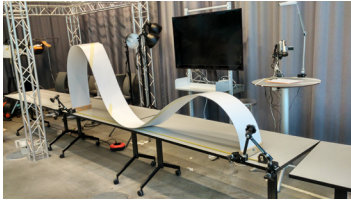
3.19 Laminated strip. The strip could not stand up under self-weight.
