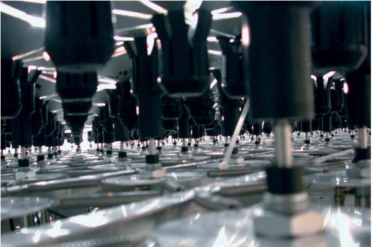
4.26 Aegis Hyposurface. View from just below the surface, showing squids and pistons.
