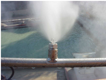
4.60 High-pressure nozzle in test setup.
