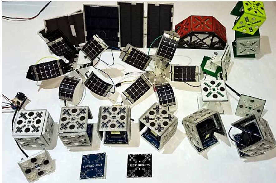
FIGURE 4.8: Collection of Modules. 5 solar panel modules, 7 servo modules, and 3 structural modules are depicted.
