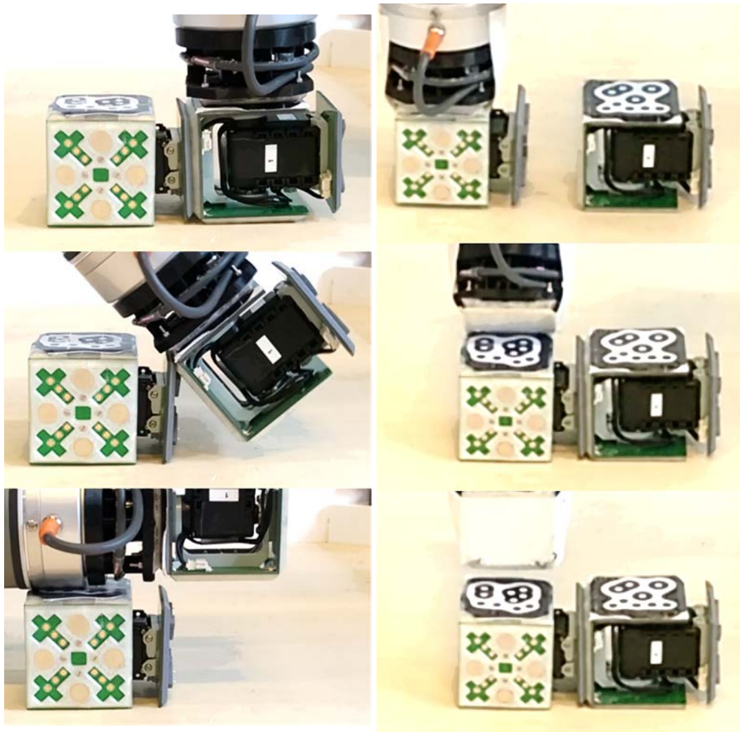
FIGURE 8.2: Assembly (left) and disassembly process (right) of modules
