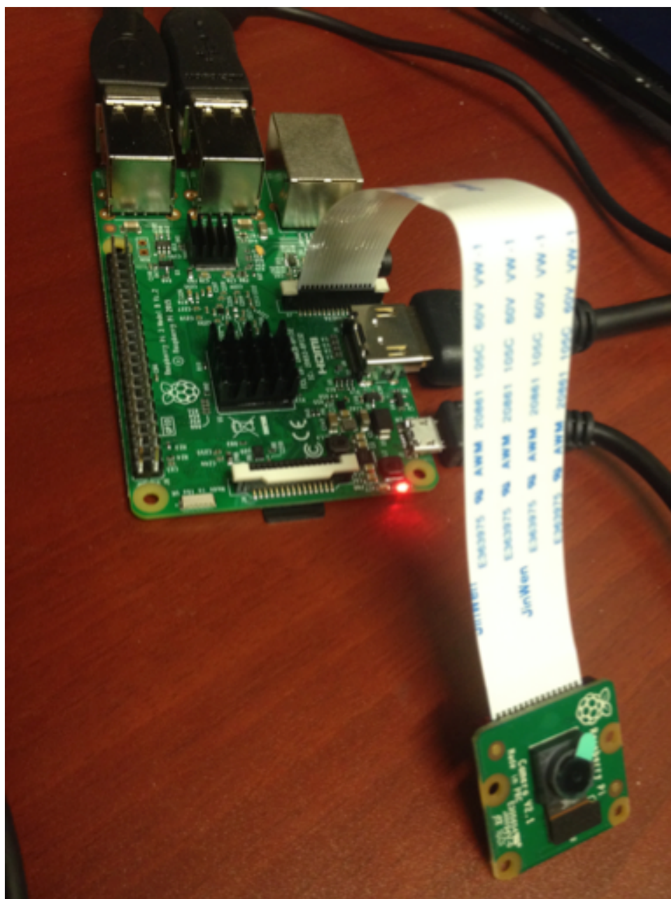
Figure 5.6.1: Using heat sinks to overclock the Raspberry Pi.
