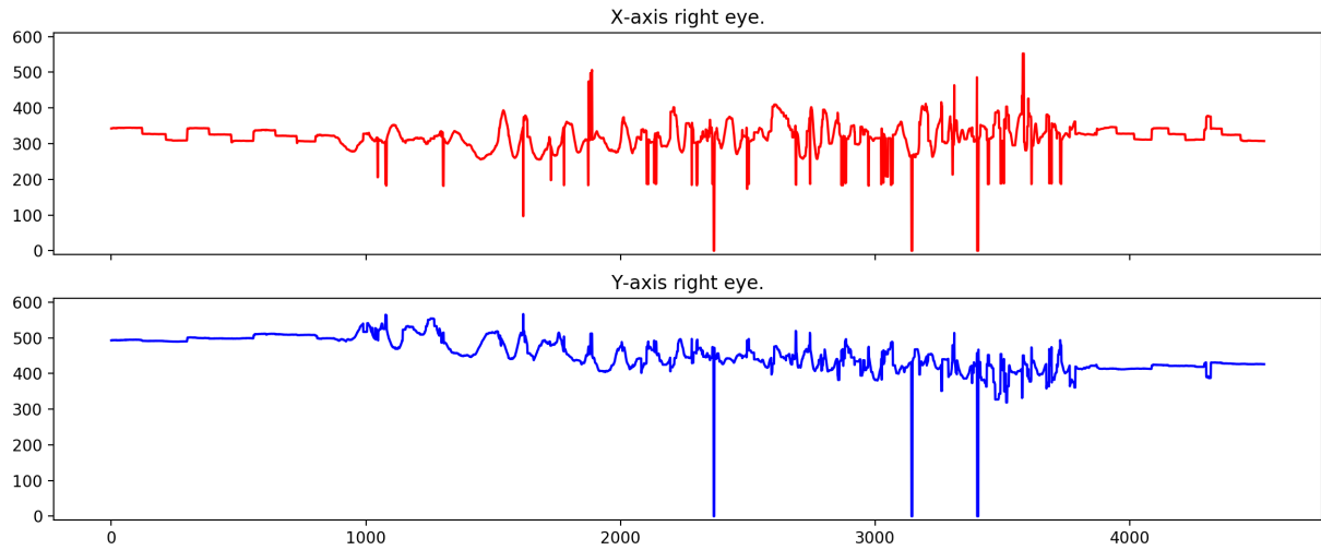
Figure 61: Influence of eye camera slippage in the eye feature detection. ( top ) X -coordinates do not change along the eye tracking session, while ( bottom ) shows a descendant curve in Y -coordinates.
