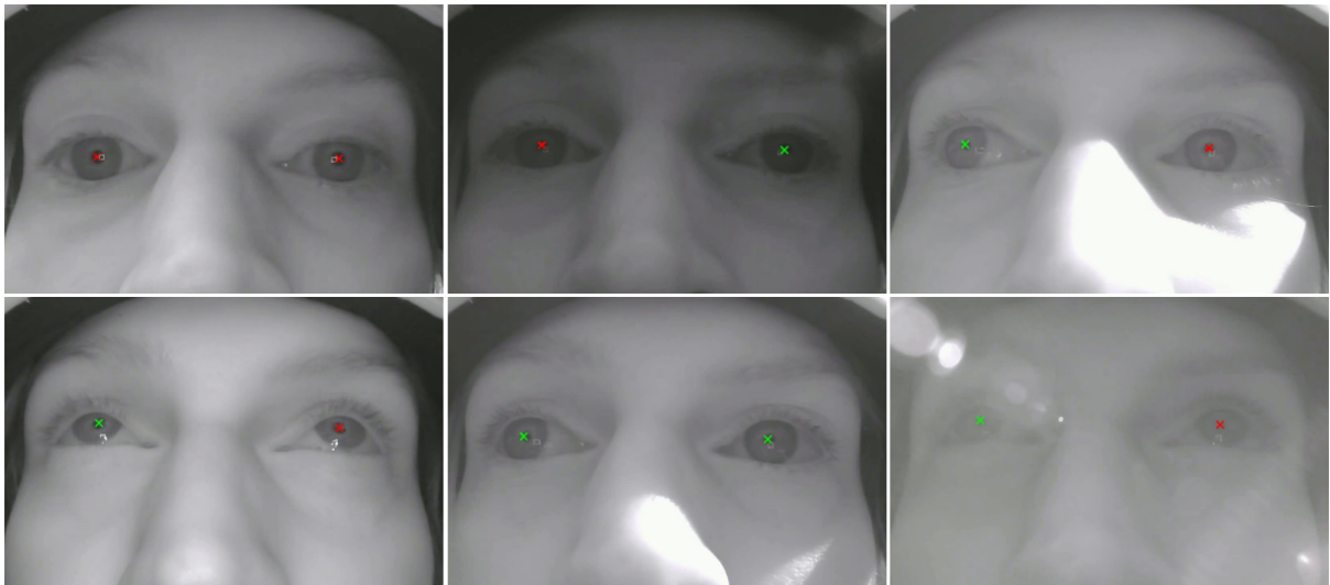
Figure 69: Pupil detection of the same athlete and trial in different illumination conditions. Red X means pupils detected correctly and green X means pupils detected using eye information as priors.
