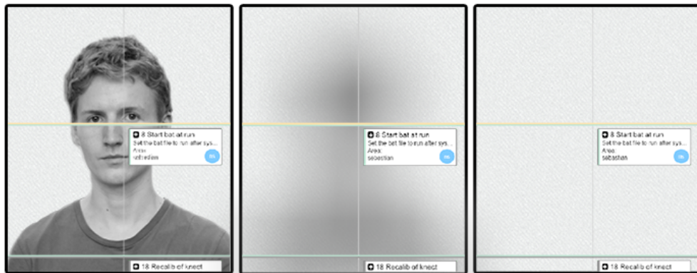
FIGURE 4.5: The dBoard uses proximity sensing to blur the video.
