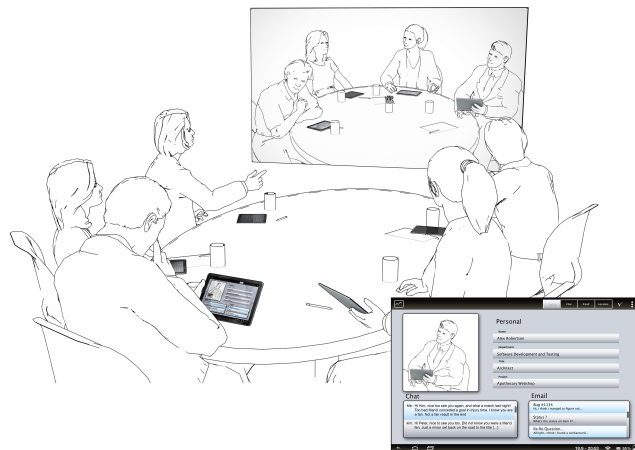
Fig. 1. SIDEBAR is a videoconferencing system supporting social engagement. This is achieved by face tracking in the video feed and by provide an interactive mirrored video feed on tablet computers, allowing users to recognize and seek information about each other, and engage in backchannel peer-to-peer chat conversations.
