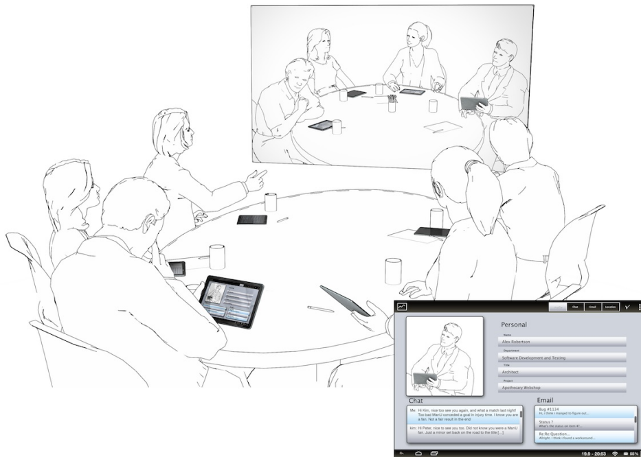
FIGURE 3.2: The SideBar system adds tablet computer for all meeting participants. Using these tablets, participants can seek out information about each other and engage in one-on-one chat conversations.
