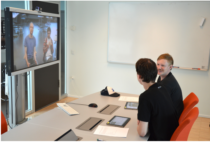
Fig. 9. Evaluation setup. A team of four persons—two at each location—is having a video meeting using SIDEBAR including the larger video display, a camera, and a tablet computer for each meeting participant.
