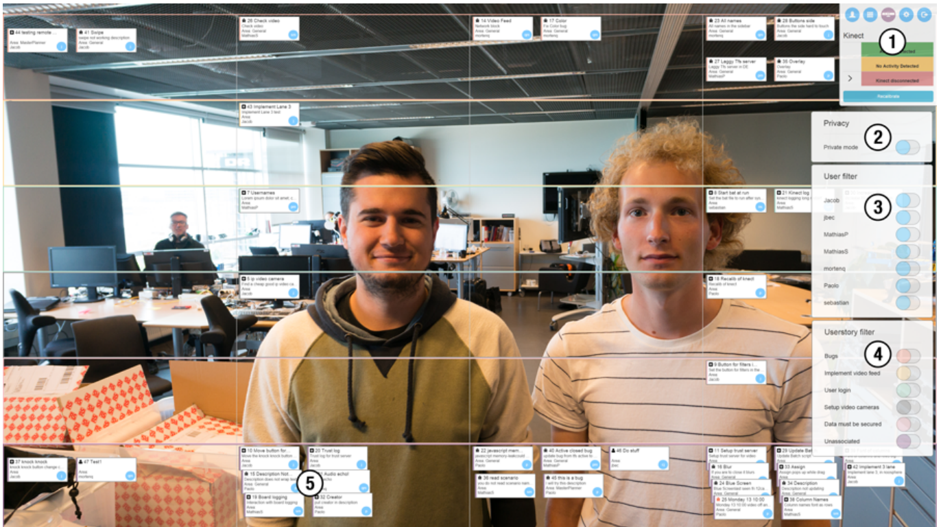
Figure 2. The user interface of the dBoard. (1) Menu, (2) Privacy menu, (3) User filters, (4) Story filters, (5) Tasks
