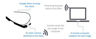
Figure 2. The system architecture of the prototype
