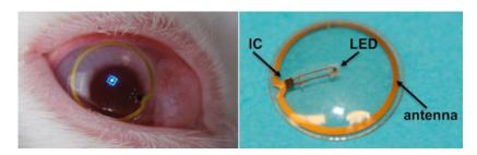
**Figure 4.5:** The right picture illustrates the first prototype of the contact lens display, and the left picture shows the contact lens in a rabbit eye [108].
