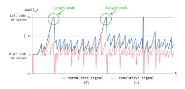
**Figure 6.3:** The blue color signal (E) is generated from horizontal eye movements in a visual search task among uni-directional moving objects that move from right to the left side of the screen. The red color signal (L) is the signal generated in the classification process. The target-peak is detected when L exceeds the  $T_r$  limit.
