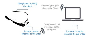
Figure 6.1: System architecture of the GlassGaze [78].
