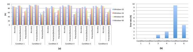
Figure 5. a) Accuracy and precision of the classification for each condition with 4 different window sizes, b) Error rate (percentage of missing targets)
