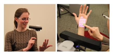
Figure 4.4: The OmniTouch system enables graphical, interactive, multitouch input on arbitrary, everyday surfaces.
