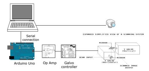
Figure 4.6: System architecture of the wearable laser pointer.
