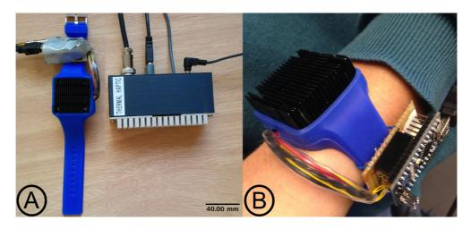
**Fig. 3** A: Wearable thermal haptic notifier system. The wearable component is on the left and the power controller component is on the right, B: Thermal haptic notifier being worn.
