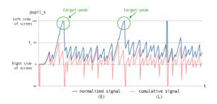
**Figure 2:** The blue color signal (E) is generated from horizontal eye movements in a visual search task among images scrolling from right to the left side of the screen. The red color signal (L) is generated in the classification process. The target-peak is detected when L exceeds the  $T_r$  limit.
