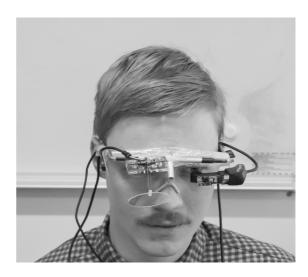
A subject wearing the eyewear setup including the gaze tracker (tracking the right eye) and a HMD on the left eye. A head tracker sensor is mounted on the right side of the Glasses frame
