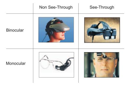
Figure 4.1: Different types of head-mounted displays [211].
