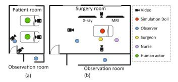
**Fig. 1.** (a) The simulation setup for the ward round scenario. The room is equipped with hidden cameras, microphones, and an observation room behind a one-way mirror. (b) The simulation surgery room for touch-less interaction and tele-presence scenarios is equipped with surgical equipments, a simulation doll connected to a monitor displaying simulated vital signs, and two large screens for displaying X-rays and Magnetic Resonance Images (MRIs).
