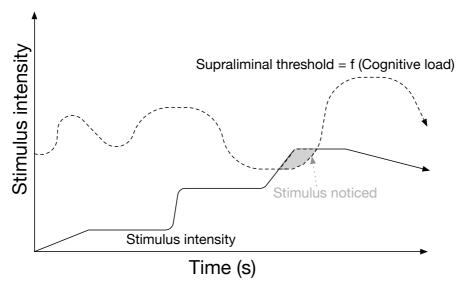
Fig. 2 Principle of self-mitigated interruption: The intensity of the stimulus (represented by the solid line) and the supraliminal threshold (represented by the dashed line), which is dependent on level of cognitive load, determines whether the stimulus gets consciously noticed. By increasing the stimulus intensity level, the likelihood of the stimulus being noticed increases.
