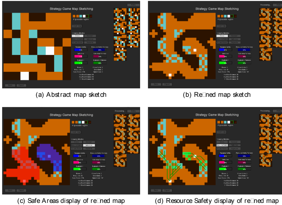
Fig. 11.6: A mockup of how iterative refining can be integrated into Sentient Sketchbook to create map sketches of varying levels of detail. The design process can begin on the abstract map sketch of Fig. 11.6a, and once the user desires they can “zoom” in to a less abstract version of the map (Fig. 11.6b) which is generated by rule-based algorithms. The same visualizations can be available on the more refined map (Fig. 11.6c–11.6d).
