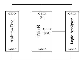
Figure 9.17: Experimental setup for measuring the time it takes to wake up from sleep initiated by a pin transition.
