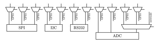
Figure 3.2: Examples of pin to functional unit routing.
