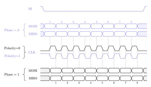
Figure 3.5: SPI line transitions. The  $\{Phase \mapsto 0, Polarity \mapsto 1\}$  configuration is highlighted in blue.
