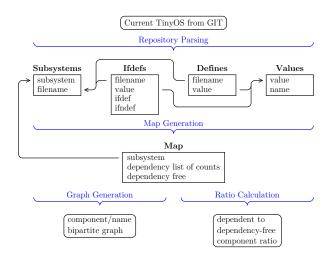
Figure 8.1: Model for analyzing the TinyOS code base. Black indicates data and blue indicates processing.
