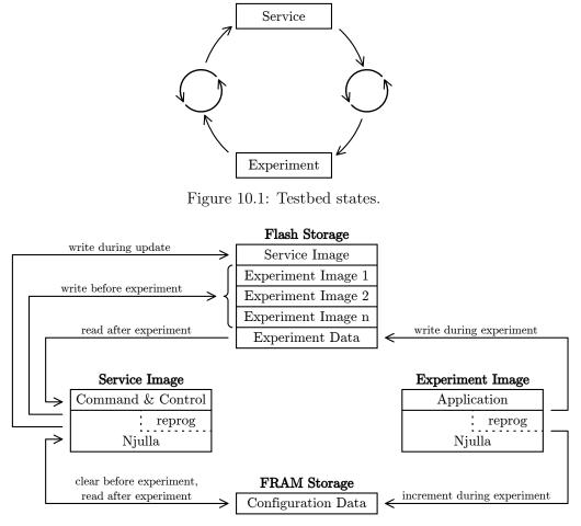
Figure 10.2: Flow of data between service and experiment images.
