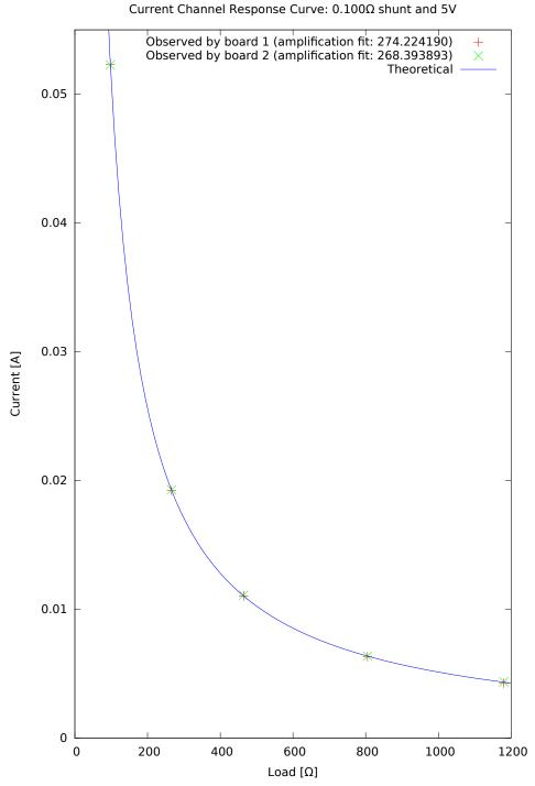
Figure B.3: Calibration result for the current channel of two PhonePower boards.
