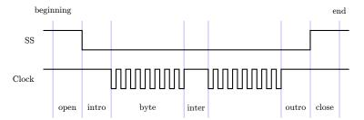
Figure 9.21: Relevant metrics for SPI benchmarking. The beginning and end marks the last and first user statement independent of the SPI communication. The interbyte time is averaged over 10 samples (11 bytes being transmitted).
