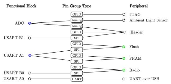
Figure 9.1: The GreenMote4 channel dependency graph. Blue nodes can only operate a single edge at a time, green nodes needs all directly connected edges to operate.
