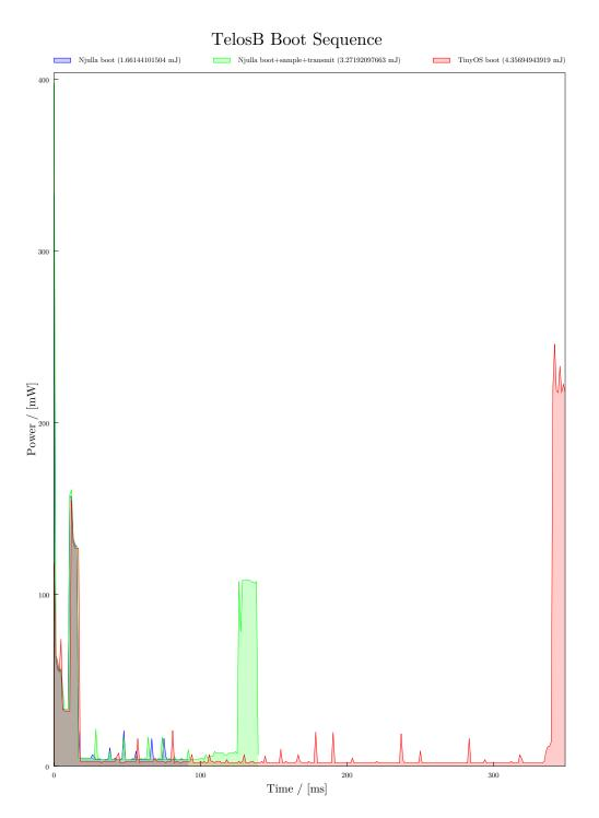
Figure 9.16: Power draw during boot for Njulla and TinyOS on the TelosB. Boot+sample+transmit for Njulla added for comparison.
