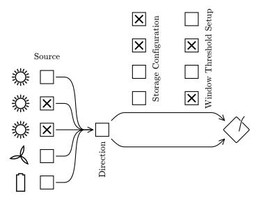
Figure 10.6: Parameters of an energy harvesting power subsystem.
