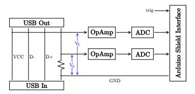
Figure B.1: Highlevel overview of the PhonePower design.
