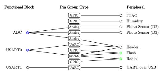
Figure 3.6: The TelosB channel dependency graph. Blue nodes can only operate a single edge at a time, green nodes needs all directly connected edges to operate.
