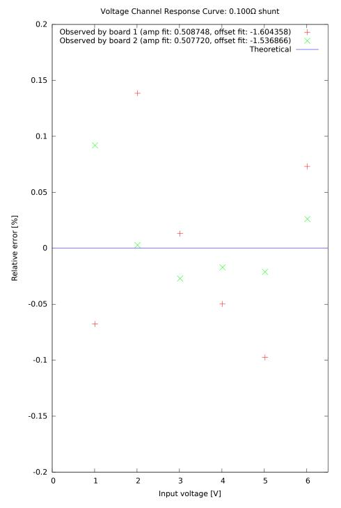
Figure B.4: Calibration result for the voltage channel of two PhonePower boards.
