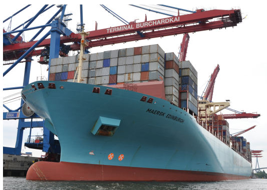
Figure 2.4: A quay crane services the post-Panamax vessel Maersk Edinburgh at the Burchardkai Terminal in the port of Hamburg, Germany.
