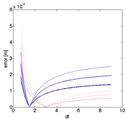
Figure 5: The effects of vertical and horizontal translations of the camera on the parallax error
