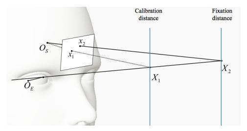
Figure 1.12: Parallax error in a HMGT
