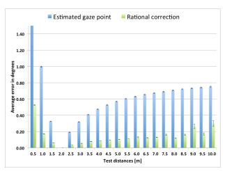
Figure 13. Average error when using the same data samples for a different subject where the camera is 5mm closer to the eye in all three dimentions.
