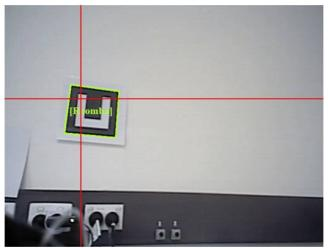
Figure 6. Visual Marker Recognition. The Hayhtham gaze tracker uses the Aforge glyph processing library (GRATF) for visual marker recognition in the scene image. This figure shows the identified marker and the user's gaze point (cross hair) in the scene image. When a subject position its gaze on a visual marker that identifies an object, the system interprets this as a pointing action and sends the subsequent recognized hand gestures to the specific object represented by the visual marker
