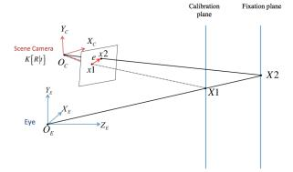
Figure 2. Parallax error in a geometrical model of a HMGT
