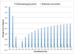
Figure 10. Average error after and before compensating for the parallax error
