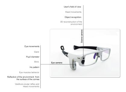
**Figure 1.9:** Many different types of information can be obtained from the eye and the scene cameras of a HMGT. Curtesy of Tobii Technologies<sup>6</sup>
