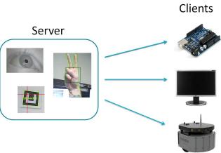
Figure 3. System Diagram. Several smart objects *clients* connect to a centralized servers that handles the gaze tracking and estimation, the visual marker recognition and the hand gesture recognition. The server dispatches the appropriate commands to a given client when a combination of gaze fixation on the object visual marker and hand gesture is detected.
