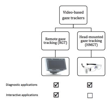
**Figure 1.1:** The application domains of the head mounted gaze trackers have been limited to the diagnostic applications. Curtesy of Tobii Technologies<sup>1</sup>
