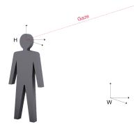
**Figure 1.8:** HMGTs that don't have a scene camera, usually estimate the line of sight in the head coordinates system (H) which can move relative to the world coordinates system (W)
