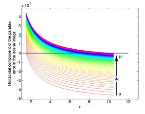
Figure 4. Translation of the function  $e_X(df)$  for a given point in the image by changing the calibration distance.
