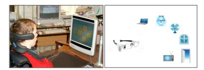
**Figure 1.2:** (left) Gaze-based interaction with one computer display using RGT (right) mobile gaze-based interaction with objects in the environment using HMGT.
