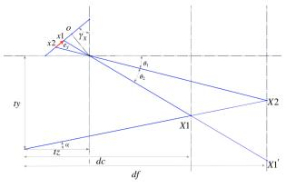
Figure 3. Vertical component of the error in the side view
