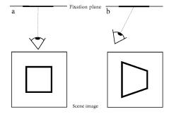
Figure 5. Viewing the fixation plane (the rectangle) from different angles and the scene images.
