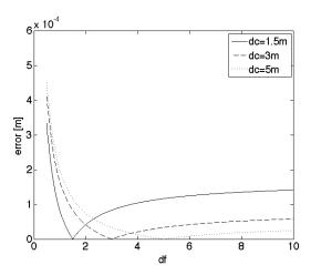
Figure 4: Changes in parallax error by changing the fixation distance
