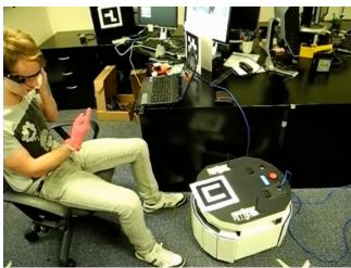
Figure 8. **System At Work.** This figure shows the user gazing at the visual marker, identifying the robot. A hand gesture is performed to transmit a movement command to the robot.
