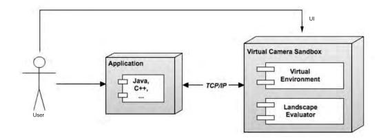
Figure 5.4: Virtual camera sandbox architecture.
