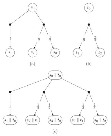
Figure 4.2: Parallel composition of  $s_0$  and  $t_0$ .
