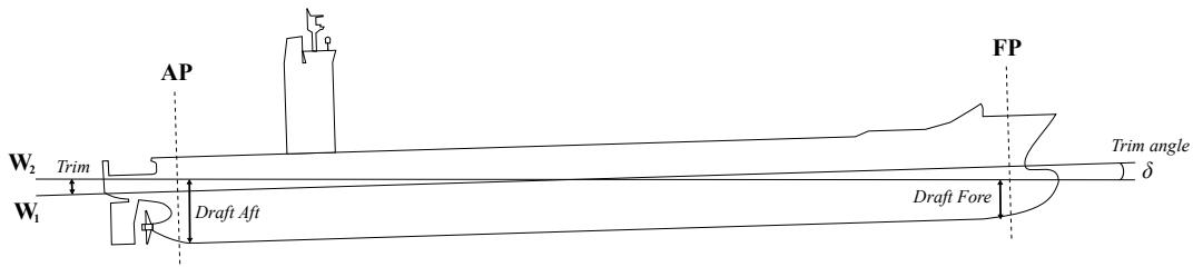
Figure 2.7: Longitudinal section of a vessel showing trim, draft and waterlines
