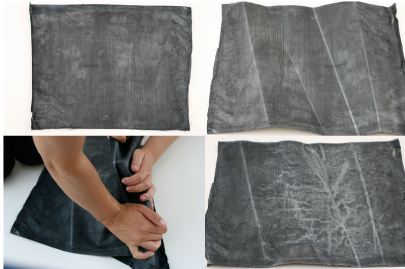
Figure 29 Black cloth coated with three layers of wood glue with well balanced abrasions.
