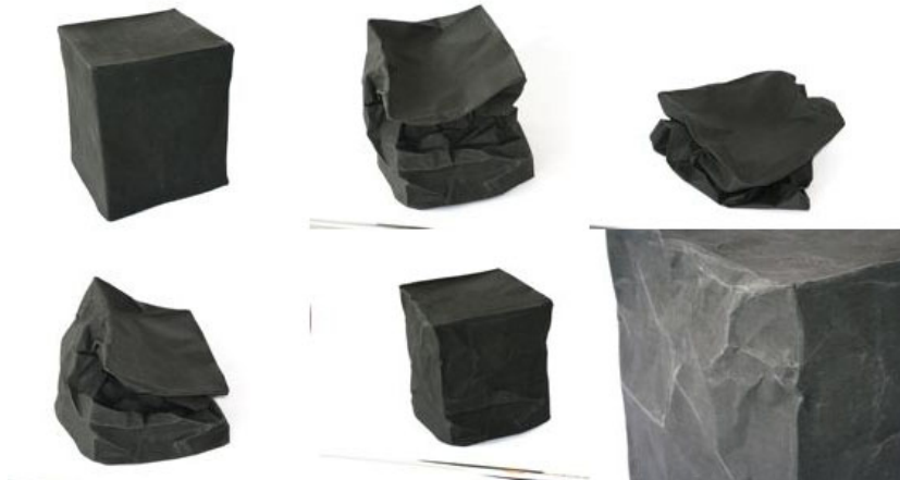
Figure 30 The lo-fi full-scale Telltale mock-up on which we, for instance, were able to text the abrasions around the edges.
