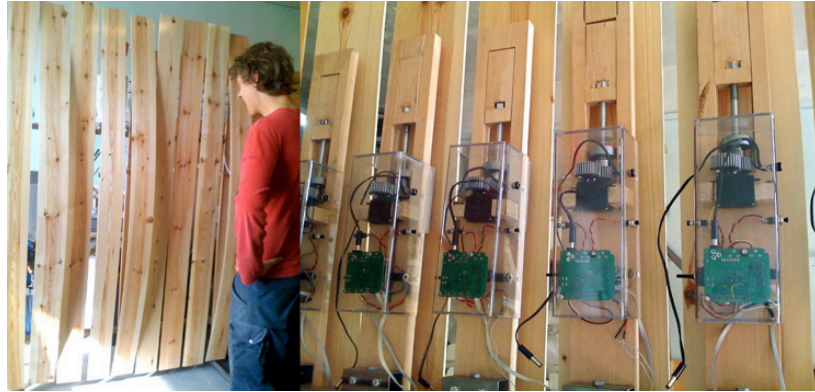
Figure 40 The first picture show the PLANKS in action. Second picture shows a close up of the computational layer and the "adhesive layer" including the motor (Unfortunately, the prototype illustrated here turned out to have a construction error and it only worked for a short while. New ones are being built.)
