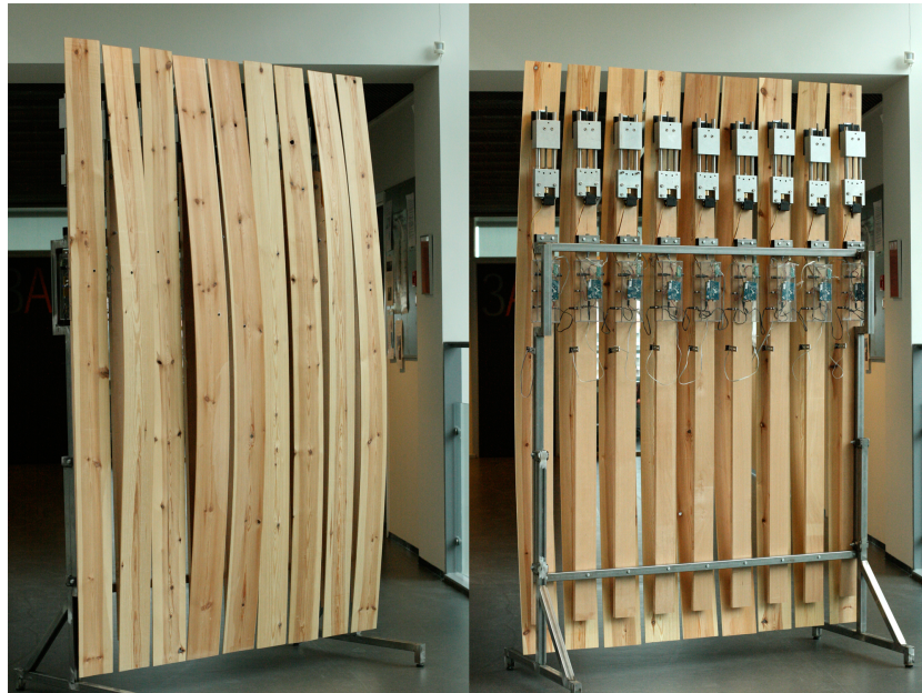
Figure 54 Nine PLANKS placed on a stand shown from the front and the back with the visible computational layer.
