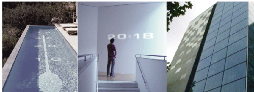
Figure 41 Chronos Chromos Concrete: the concrete can change color in response to a computer's output. The composite is made from thermo chromatic ink, nickel chromium wire, computers, and concrete (Ibid.).
