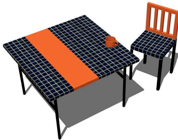
Figure 56 An example application of a material, which is physically dispersed but thermodynamically coherent. For instance, the warmer the cup is the warmer the back of the seat and the area of the table gets and vice versa .
