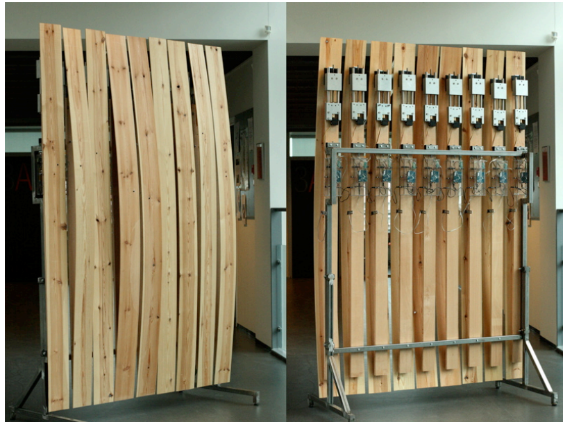
Figure 42 PLANKS: planks of pinewood flex as a reaction to sonic activity in their vicinity. Each plank work individually and can thus be used for a variety of different purposes such as wall panels or doors. The composite is made from pine planks, motors, microphones, and an Arduino computer (Ibid.).
