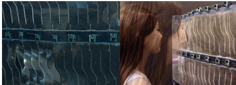
Figure 13 Living Glass is a polymer glass substitute that opens and closes in response to human presence to control the air quality in the room. (Courtesy of The Living)
