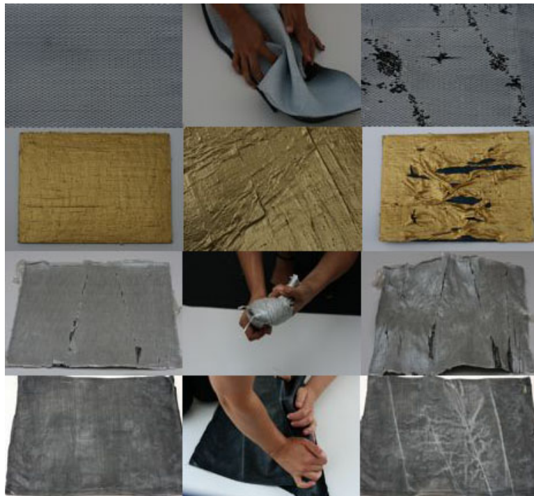
Figure 48 Experiments with material expressions for Telltale. By applying a fragile layer within the composite or an added surface treatment, we were able to explore the range of materials expressions at different points in a process of wear and tear
