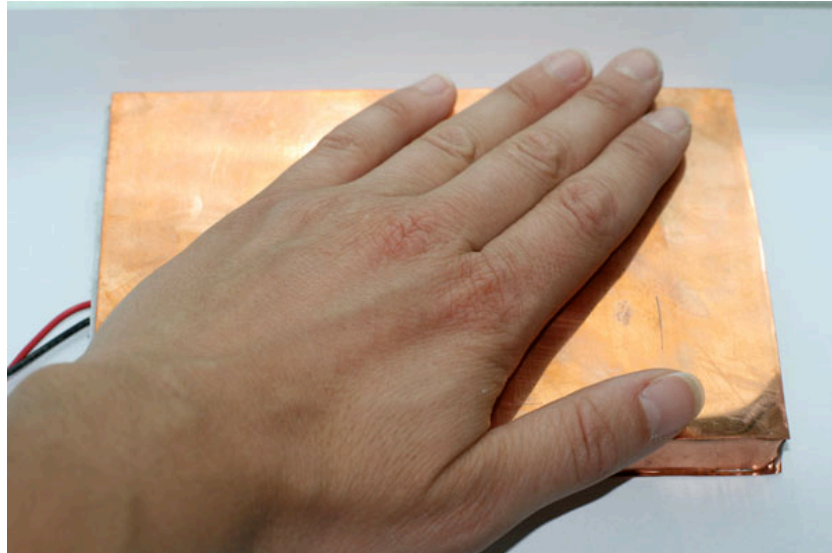
Figure 23 The heat from a hand is enough to turn the composite cold within few seconds.
