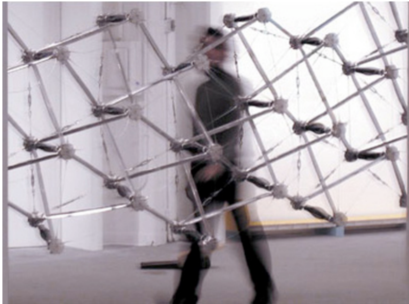
Figure 35 A prototype of an actuated tensegrity structure, courtesy of oframBFRA
