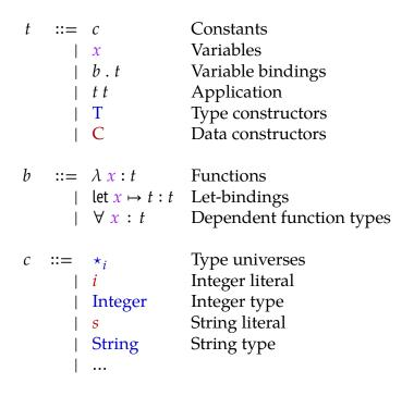
Figure 4.2: The grammar of terms t, binders b, and constants c in Idris's core language TT.
