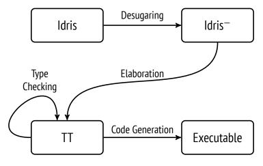
Figure 4.1: The Idris compilation process.
