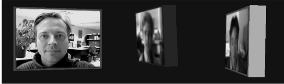
Figure 3.2: GAZE-2 scales and rotates video to convey gaze direction. The focus of the participants are on the person on the left. Image taken from [26].
