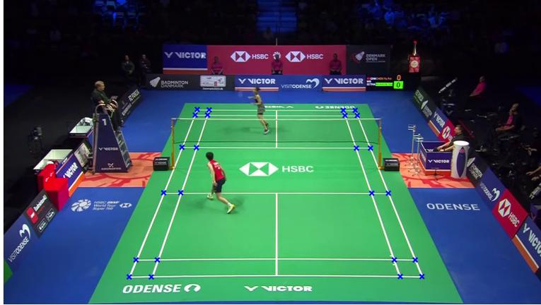
**Figure 4.2:** Using the known dimensions of a badminton court, a homography transformation is calculated to map image coordinates to court coordinates, facilitating the estimation of court positions and camera parameters. Corresponding points between the image and the court are used to compute the transformation.
