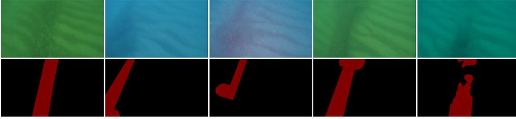
Figure 4.6: SubPipe images. Top: Original raw images; Bottom: Manually annotated Ground-truth
