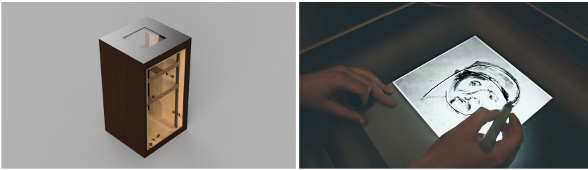
Fig. D.3: The left image is a render of the prototype with the sides open, so the inner structure can be seen. The image to the right shows a user interacting with the drawing interface.
