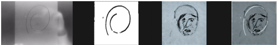
Fig. E.3: Inferring a Munch-like sketch from a hand-drawn line. From left to right: 1) infrared webcam image from beneath the drawing surface. 2) The cleaned input image. 3) The synthesized sketch. 4) A composite image of the input image over the synthesized sketch that is output as a projection on the tracing paper.
