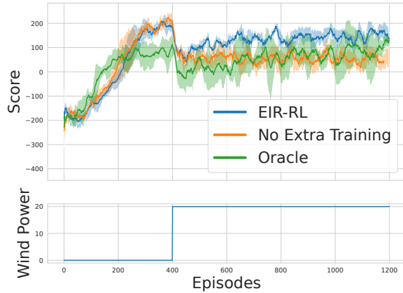
Figure 6.8: Lunar Lander: PPO Training Curves. Means and standard deviations over 5 different PPO runs. Plotted is the moving average of the objective (non-evolved) scores of the latest 20 episodes. The EIR-RL is able to recover most of the performance when strong wind is applied.
