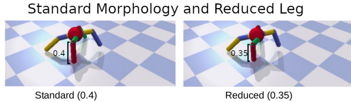
Figure 4.2: Robot Environment. Right: The standard morphology that the models were optimized for. Left: An example of the most severe leg reduction done to a leg to test robustness. The lower part of the leg was reduced from 0.4 to 0.35. In this figure, the reduction was done to the red part of the leg in the foreground of the image.
