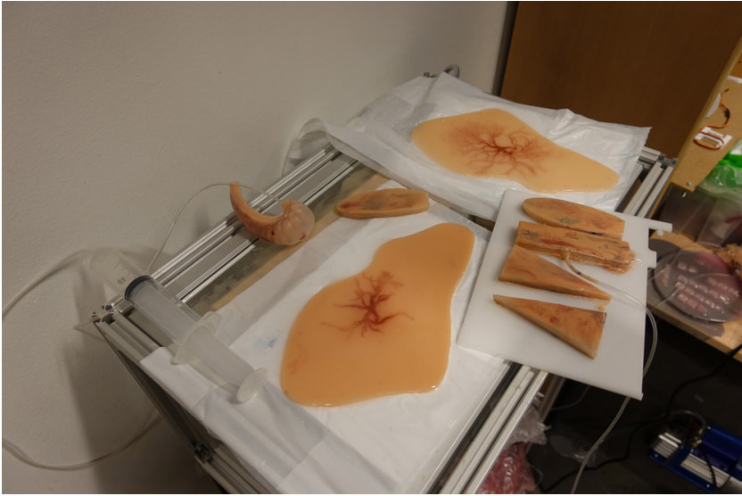
Fig. 43. Flesh-like silicone parts.
