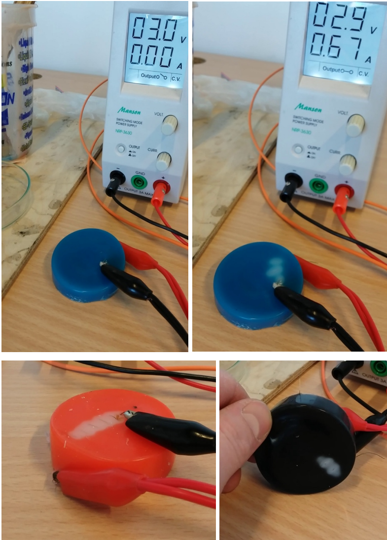
Fig. 40. Silicone colored with thermochromic pigments heated with Kanthal thread.
