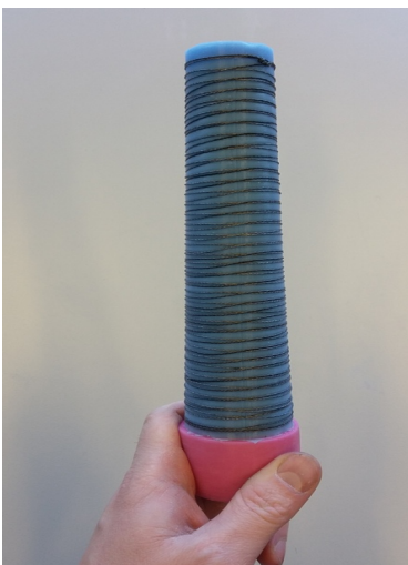
Fig. 35. The fishing line is wound around the tentacle from the top to the bottom in the opposite direction of before and fixed with a knot and epoxy glue at the bottom. The overlaps between the windings are aligned to be vertically parallel on opposite sides of the tentacle, and the distance between the windings adjusted with the 3D printed guide.
