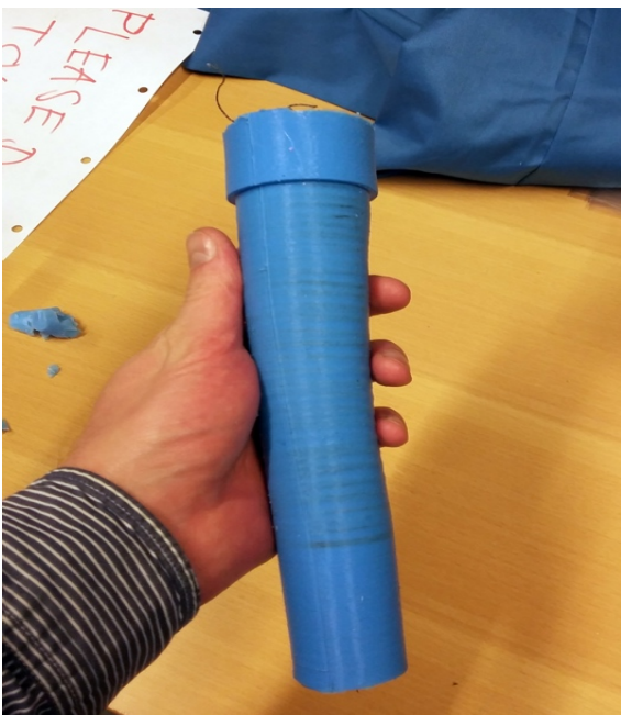
Fig. 37. After 24 hours of curing, the tentacle can be removed from the mold and the bottom and tubes can be attached.
