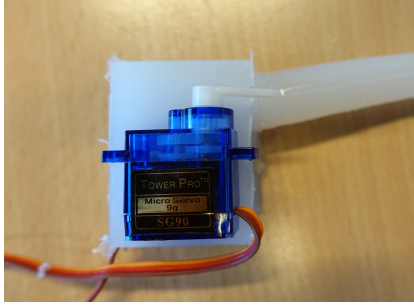
Figure 5: A servo motor placed on top of a servo enclosure to illustrate where the motor and the servo arm are located inside the enclosure. (© Jonas Jørgensen. Photo: Jonas Jørgensen.)
