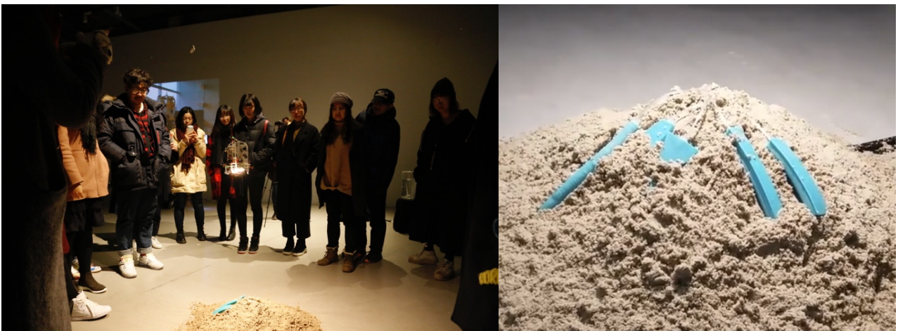
Fig. 24. Beyond Digital Towards Biological (2017). Left: Visitors watch as the hanging robot interacts with the group of earthbound green soft actuators. Right: close-up showing the green soft actuators in the pile of sand (the microcontroller, pumps, valves, and light sensor were hidden inside the pile).
