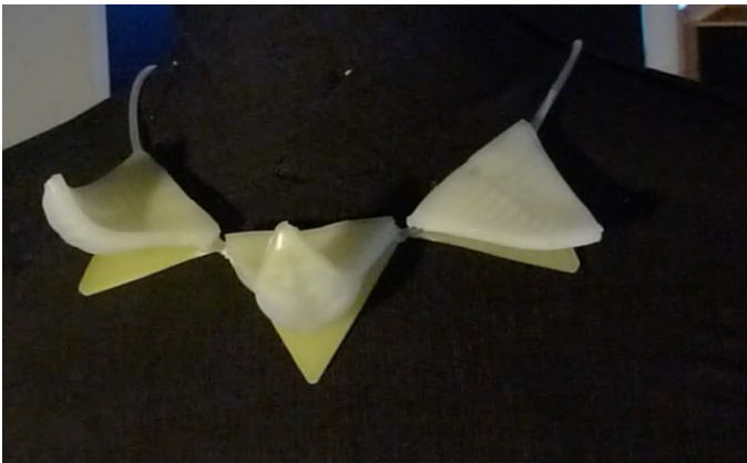
Fig. 14. Caroline Yan Zheng, Wear the heart on the sleeves (2017). Prototype of interactive soft robotic necklace that responds to a heartbeat sensor.
