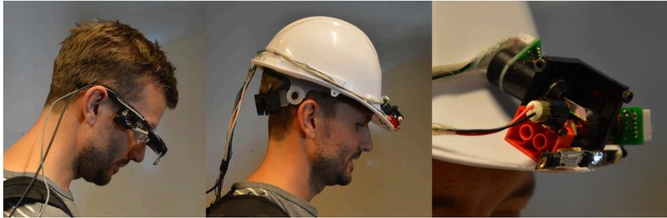
**Figure 4.7:** *The right picture illustrates a closer view of the galvo scanners, the middle image shows a user wearing the helmet-mounted motorized laser pointer while the left picture shows a user with the HMD [83].*
