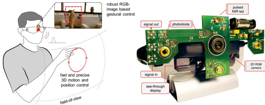
**Figure 5.2:** *Mime can be added as a peripheral component to eyewear computers for gesture-based interaction [39].*
