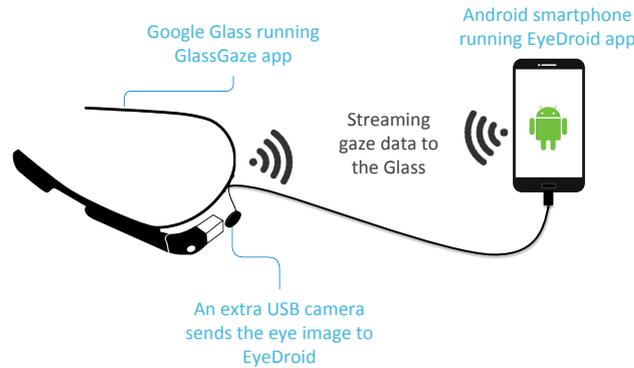
**Figure 6.2:** A schematic view of the EyeDroid system architecture.
