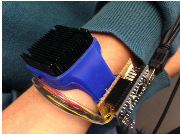
**Figure 7.1:** *Wearable thermal haptic notifier system [27].*
