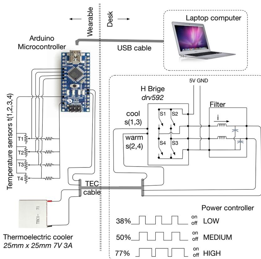
**Fig. 4** System architecture diagram. The components of the wearable device are on the left side (Thermoelectric cooler, Arduino Nano, and 4 thermistor based temperature measurements). A simplified h-bridge is shown in the power controller block.
