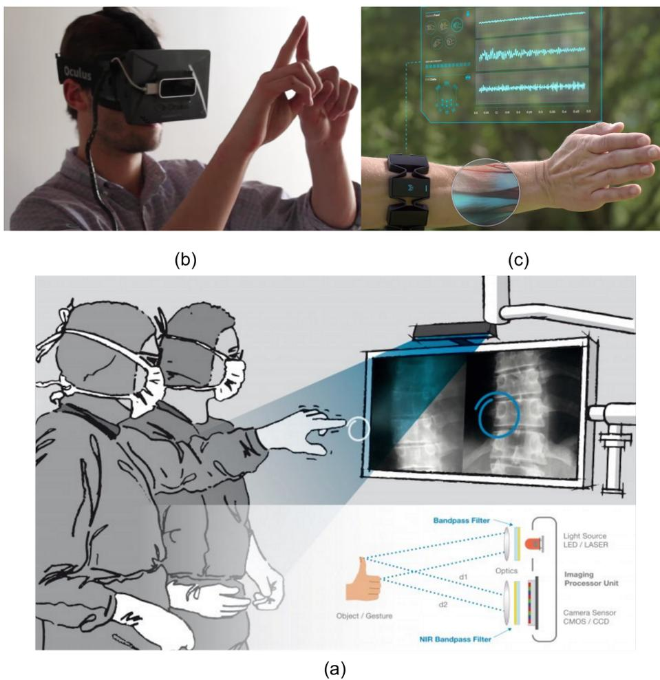
**Figure 5.1:** a) Opticsbalzers TOF camera for gesture recognition in surgery rooms, b) Leap Motion sensor for interaction with virtual reality applications, and c) Myo sensor detects hand gestures by analyzing electrical signals from muscles (EMG).
