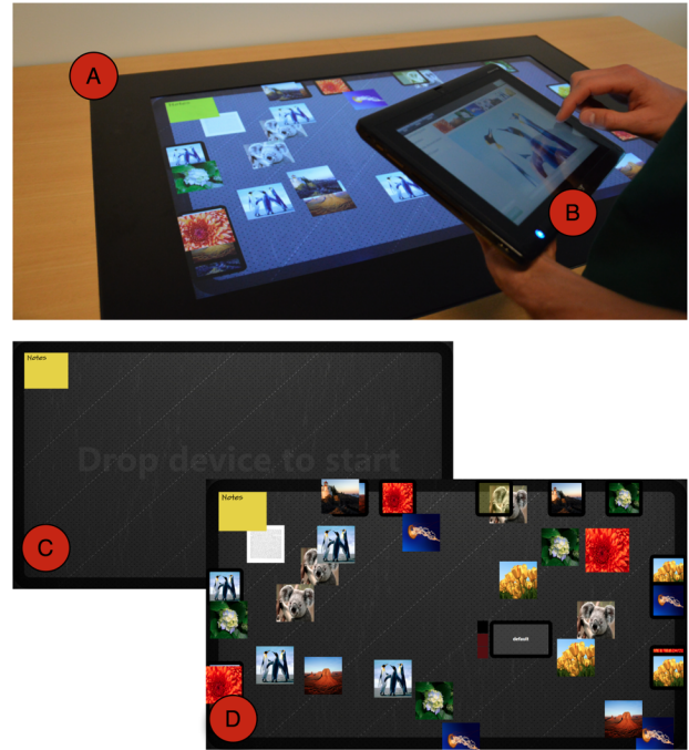
Figure 6: The public tabletop (A) connected to a tablet (B). The user walks up to an empty public interactive table (C) and simply places his device on top of the tabletop. The table will recognize the device and use the discovery to find and connect to the activity manager of the tablet. All resources related to the active activity on the mobile device are deployed on the interactive surface (D). When the user switches between activities, the interactive desk is repopulated with resources related to that activity. Users can utilize the desk to exchange, modify or manage files and resources. Additionally, the system allows the user to redirect input from the table, thereby providing remote control over the surface.
