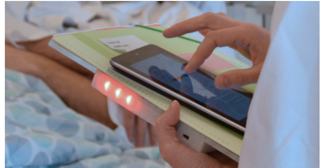
Figure 1. A Hybrid Patient Record (HyPR) device augments the paper patient record with color configuration and location tracking, while allowing clinicians to pair a tablet which shows the digital information associated with the paper record.
