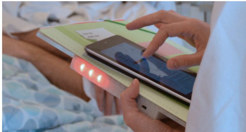
Figure 5.22: A Hybrid Patient Record (HyPR) device augments the paper patient record with color configuration and location tracking, while allowing clinicians to pair a tablet which shows the digital information associated with the paper record.
