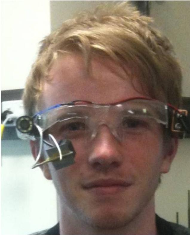
**Figure 5. Low Cost Gaze Tracking Glasses On a Subject.** This figure shows how the low-cost head-mounted gaze tracking system looks while being used by a subject.
