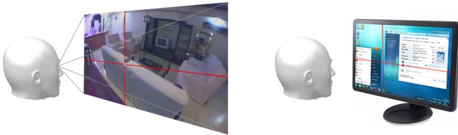
**Figure 1.7:** (left) RGT estimates the gaze point in a fixed two-dimensional space e.g., computer display. (right) In contrast, HMGT estimates the gaze in the user's FoV.
