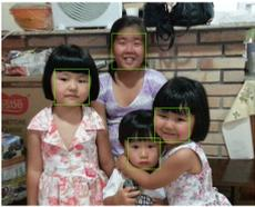
Figure 3: Faces detected using the Viola-Jones algorithm.
