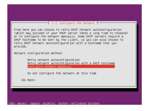
Set up static IP for the (public) network interface:
