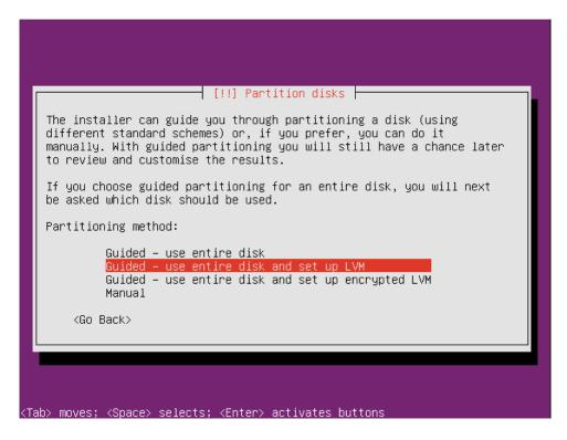
In our case, we have only one large disk, and we would just partition it using default options. If having several disks, we could choose another way of partitioning, for the sake of performance or redundancy.
