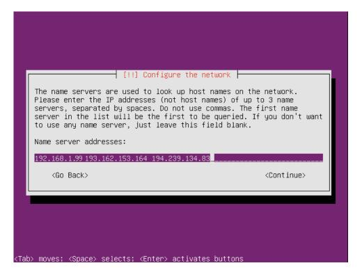
The first one to be contacted would be the first one from the list. In our case it is the local server's address (192.168.1.99), since we will install DNS server on this server later on.
