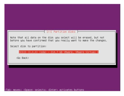
If the disk was used before, having some partitions on it, we would be prompted to overwrite the old configuration, warned that we would lose all the data saved on the disk.
