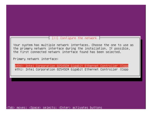
The installation automatically configures this network interface for DHCP:
