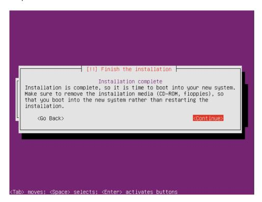
Make sure that you un-mount / take out the installations media (CD), to prevent the system booting again into installation. If that happens, you just cancel the installation, take the media out, and recycle the machine – no damage to the installation is done.
