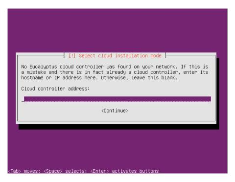
Choosing the components to be installed on the first server – we install Cloud Controller and WS3. This is a design choice, since in our case we want to try scale out possibilities, and we are initially separating cloud and cluster components. We choose the components common for the whole cloud:
