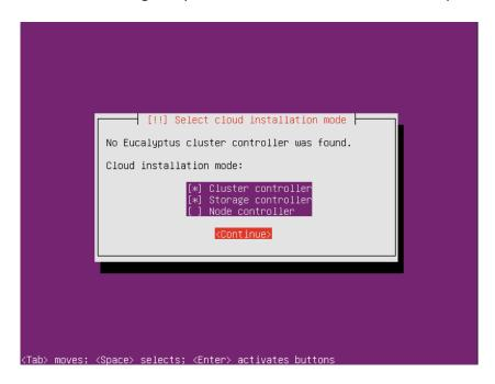
(If the installation complains that it cannot find a CLC or WS3, check the networking before going on!)
