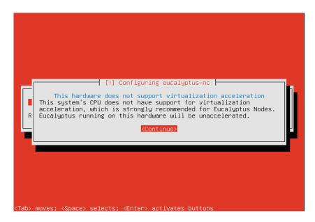
(In our case, we get the error since we are installing UEC inside a virtual machine, where VT extensions are not supported)
