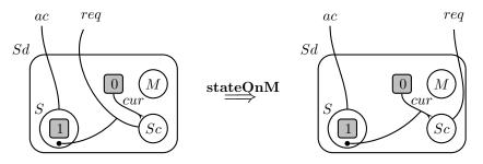
In this rule, we see the first simple example of the usage of binding in a reaction rule. We analyze the gain in using a binding bigraph reaction rule in this case, by asking: Could we just have let the *cur* link be an outer name, instead of a local link to a particular site?
