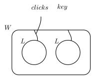
Registering a listener as an event-handler, for a particular kind of event associated with some component, amount to connecting a port associated with that event of the component (e.g., the *key* port for a window) with the port of the listener. This will allow us to let a single listener handle different kinds of events.
