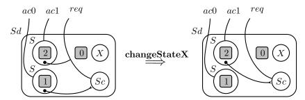
Note that this rule does not leave out the possibility of having exclusive state diagrams with one or zero S-nodes. Such state diagrams make sense, if we allow state diagrams to change dynamically – by allowing reaction rules to add or remove S nodes.
