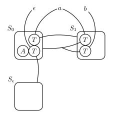
We encode the input sequence as a linked list using atomic controls *i* with arity 3. The first two ports are linked to the next and previous elements of the list, respectively, and the third port is linked to an inner name representing a symbol of  $\Sigma$ . Finally, we append the symbol  $\epsilon$  to the input sequence. Altogether, the input sequence *aaba* becomes the following bigraph.
