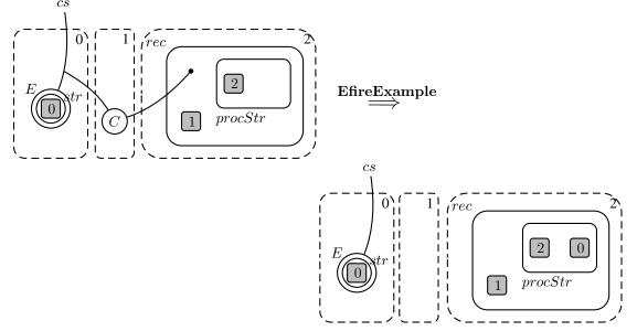
In the example rule given above, we state the intended semantics of a command request, connected to an event containing a *str* component, upon a *rec* component with a *procStr* subcomponent. We could specify another rule, allowing the same component to react in a different manner, when associated with a command linked to another kind of event.
