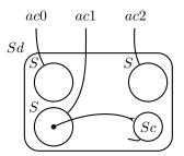
The arity of an S-node is 1, allowing us to associate a component with each state in a state diagram. This will allow us to let behavior of the system *depend* on state (see the end of this section). This port will be linked to a discrete outer name in all rules except **fireStateCond**.
