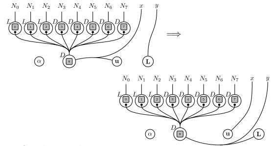
In the  $\beta$  part of the computation, nodes are updated and next states are reset to u. We will need to have 4 reaction rules, one for each of the 4 combinations of previous and next state. We give only the one in which a dead cell becomes live.
