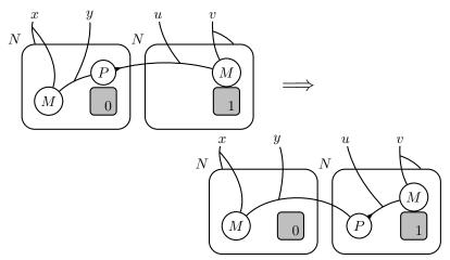
Now all we need are rules for broadcasting packets to machines that have not been located. If we satisfy ourselves with modeling a 3-way switch, writing such a rule is straightforward. Instead, we give rules for broadcasting on an arbitrary number of networks. First, we recognize when to broadcast. We mark packets that need broadcasting as such by enclosing them in a control B of arity 0.
