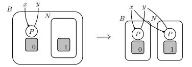
Once the B node contains no more networks, the packet have been broadcast. We can now safely remove the B node and its copy of the packet.
