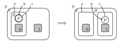
The copying itself is a recursive process, transmitting the packet on one network, while recursively copying the packet onto the remaining networks.
