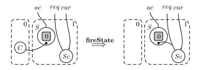
We would also like to be able to let behavior of the system *depend* on state. One way of modeling this is by associating to each S node a component, and adding the following reaction rule:
