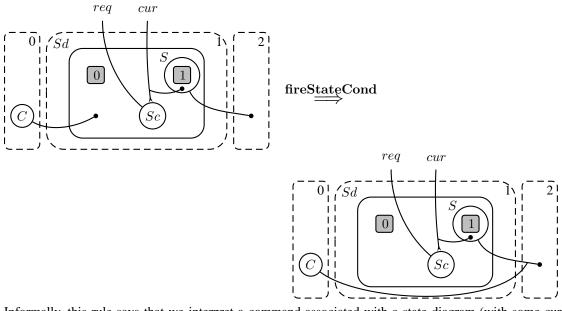
Informally, this rule says that we interpret a command associated with a state diagram (with some current state), as a request for issuing a command to the component associated with the current state. (Note, that the rule works for both kinds of state diagrams, but again we have an inherent nondeterministic choice, if there are multiple current states.)
