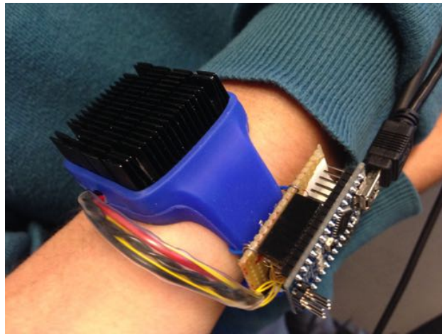
Figure 7.1: Wearable thermal haptic notifier system [29].
