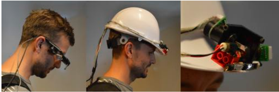
Figure 4.7: The right picture illustrates a closer view of the galvo scanners, the middle image shows a user wearing the helmet-mounted motorized laser pointer while the left picture shows a user with the HMD [84].
