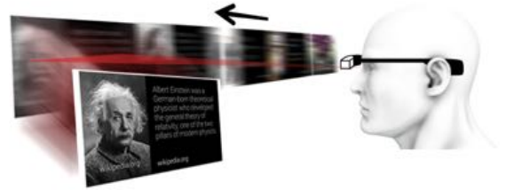
Figure 1: A right-to-left fast scrolling menu on a head-mounted display where it stops on the content that has attracted the user's visual attention (Einstein's picture)
