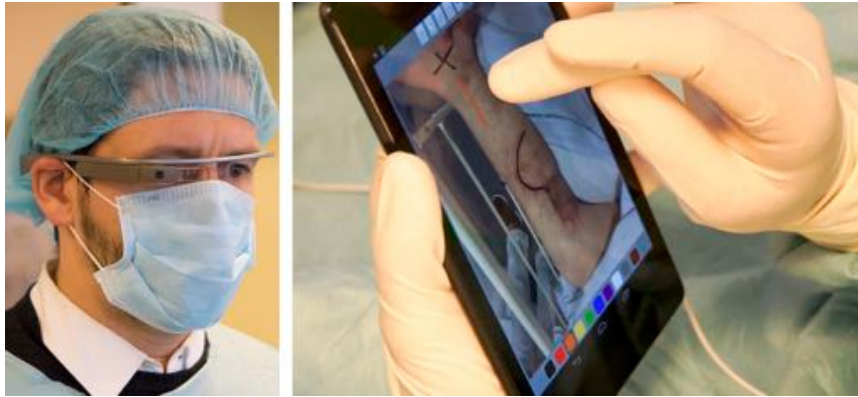
Figure 3.7: A remote surgeon (right picture) uses a tablet computer to provide guidance to the local surgeon (left picture). The local surgeon sees the visual guidance on the HMD in real-time [83].
