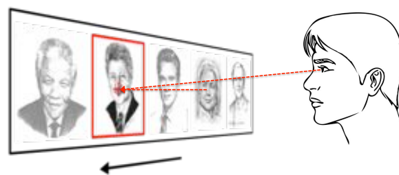
Figure 1. EyeGrip technique to detect an object of interest among horizontally moving images
