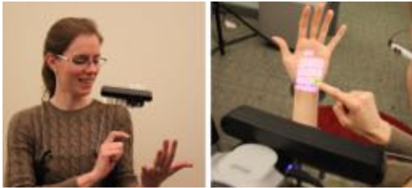
Figure 4.4: The OmniTouch system enables graphical, interactive, multi-touch input on arbitrary, everyday surfaces.
